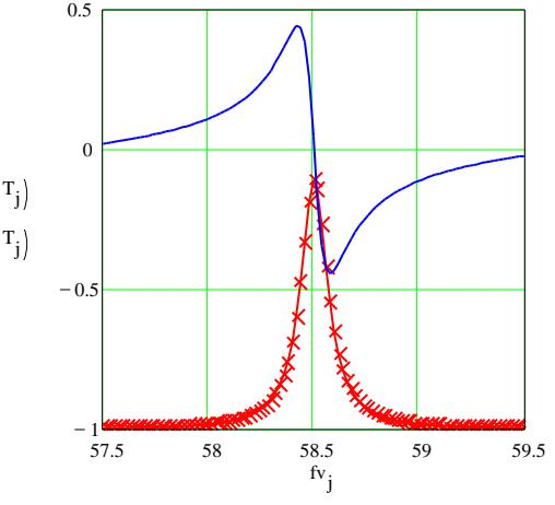
Calc. current and voltage along current strap, for specified f and R -
